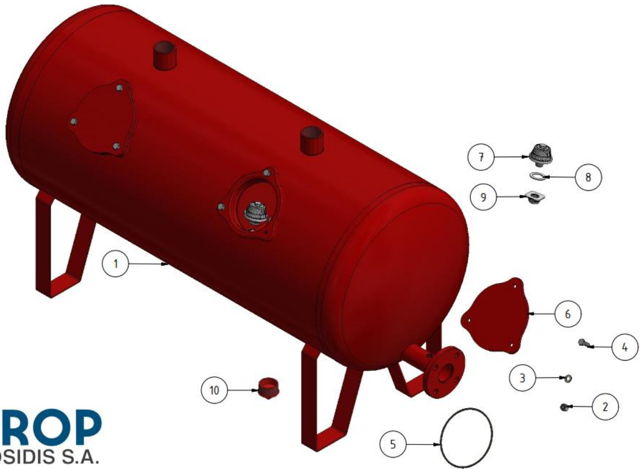
05-08-212 Dual chamber sand media filter series XDC 2'' with false bottom
